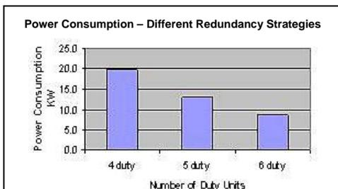
The second test had five units operate at reduced speeds and the sixth unit off. The third test had all six units operating at reduced speeds. Once again the BMS was used to maintain a constant static pressure in the raised floor. With full air flow operating, the static pressure set point was 0.03" w.c..
